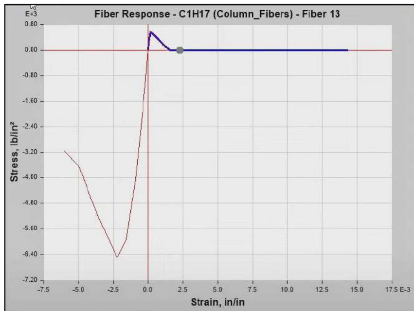
Figure (4.20): Stress-strain curve for fiber 13 of column C1
