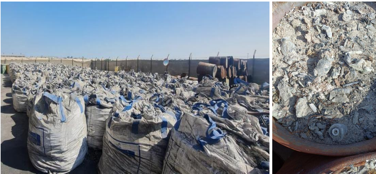
Figure 4.27 Generated bottom ash in BWTC, pictures taken during the site visit.
