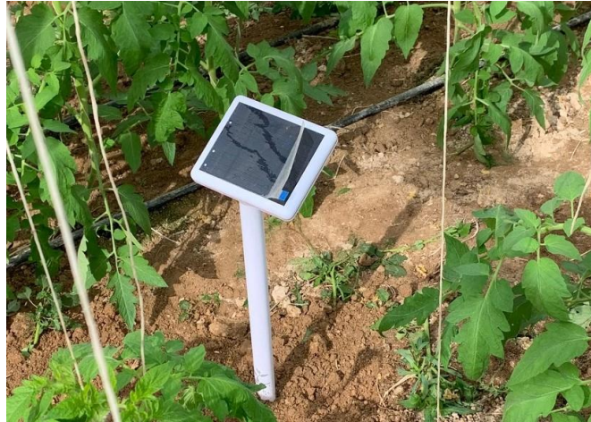
Figure (5.4): The Pycno soil sensor positioned in the selected farm.
