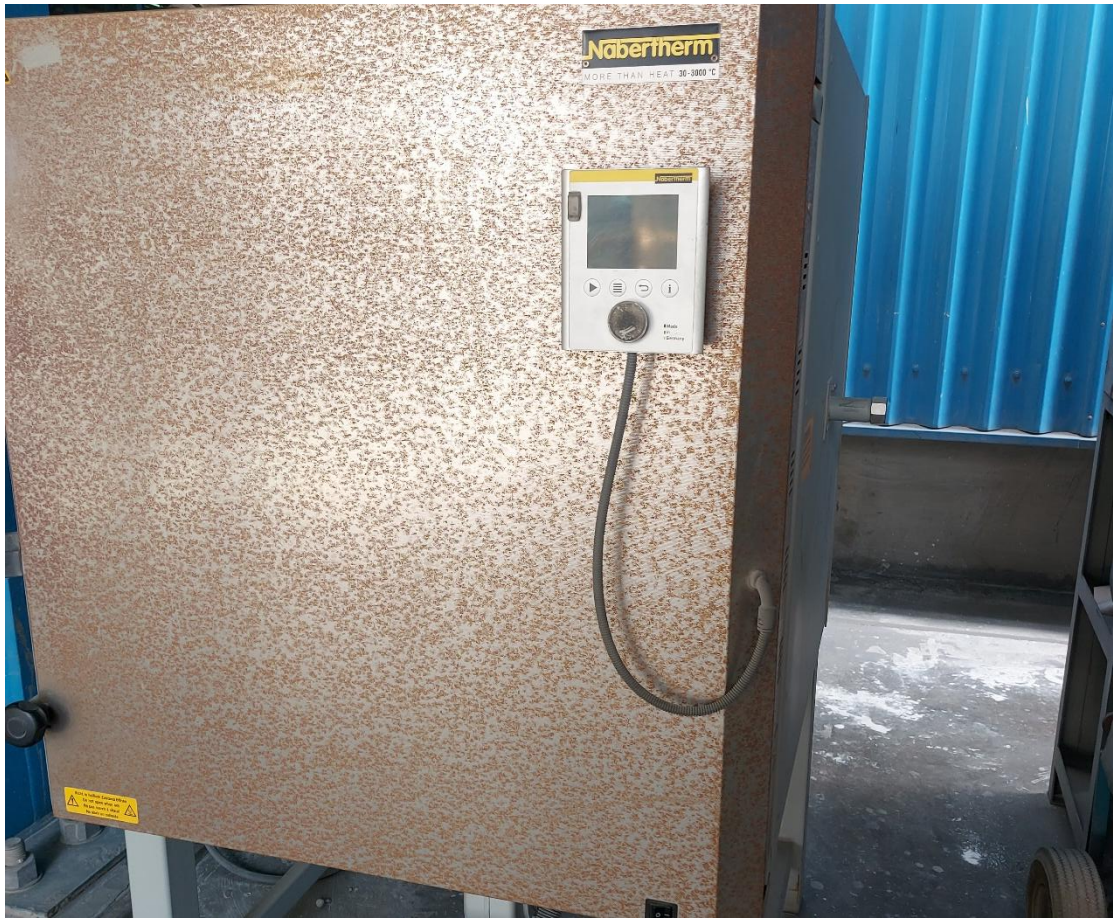
Figure 3.2: The electric furnace used in heat treatment.
