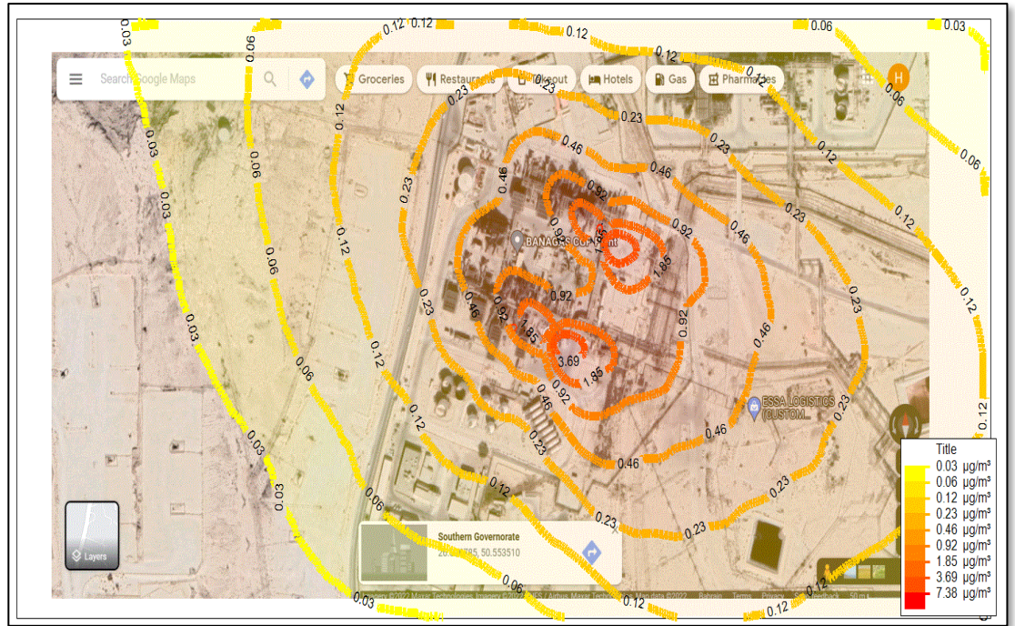
Fig.27: Contours of H 2 S mean concentrations ( \mu\text{g}/\text{m}^3 ) at 3 meters height above the ground- drain pots
