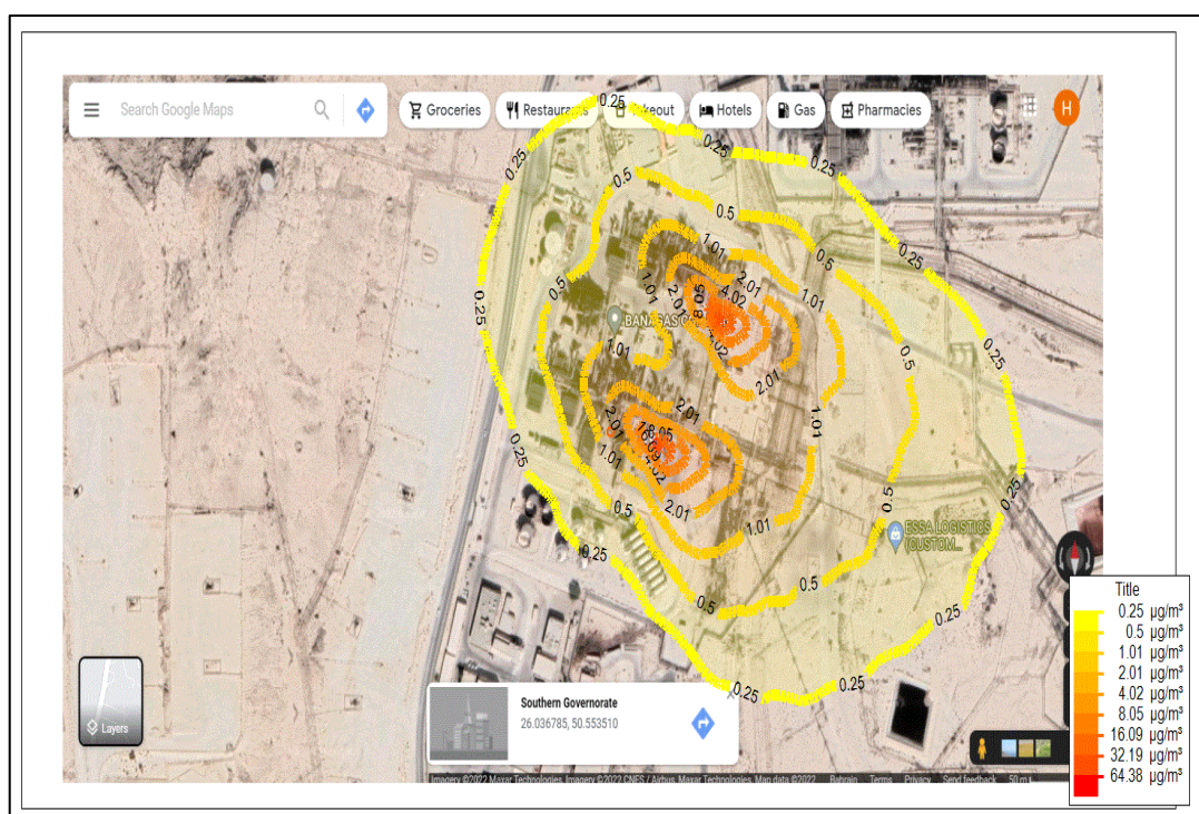
Fig.26: Contours of H 2 S mean concentrations ( \mu\text{g}/\text{m}^3 ) at 1.8 meters height above the ground- drain pots
