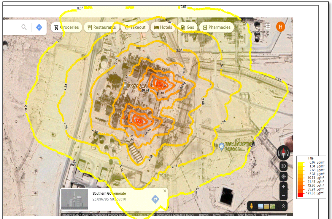
Fig.29: Contours of H 2 S daily maximum concentrations (µg/m 3 ) at 1.8 meters height above the ground- drain pots
