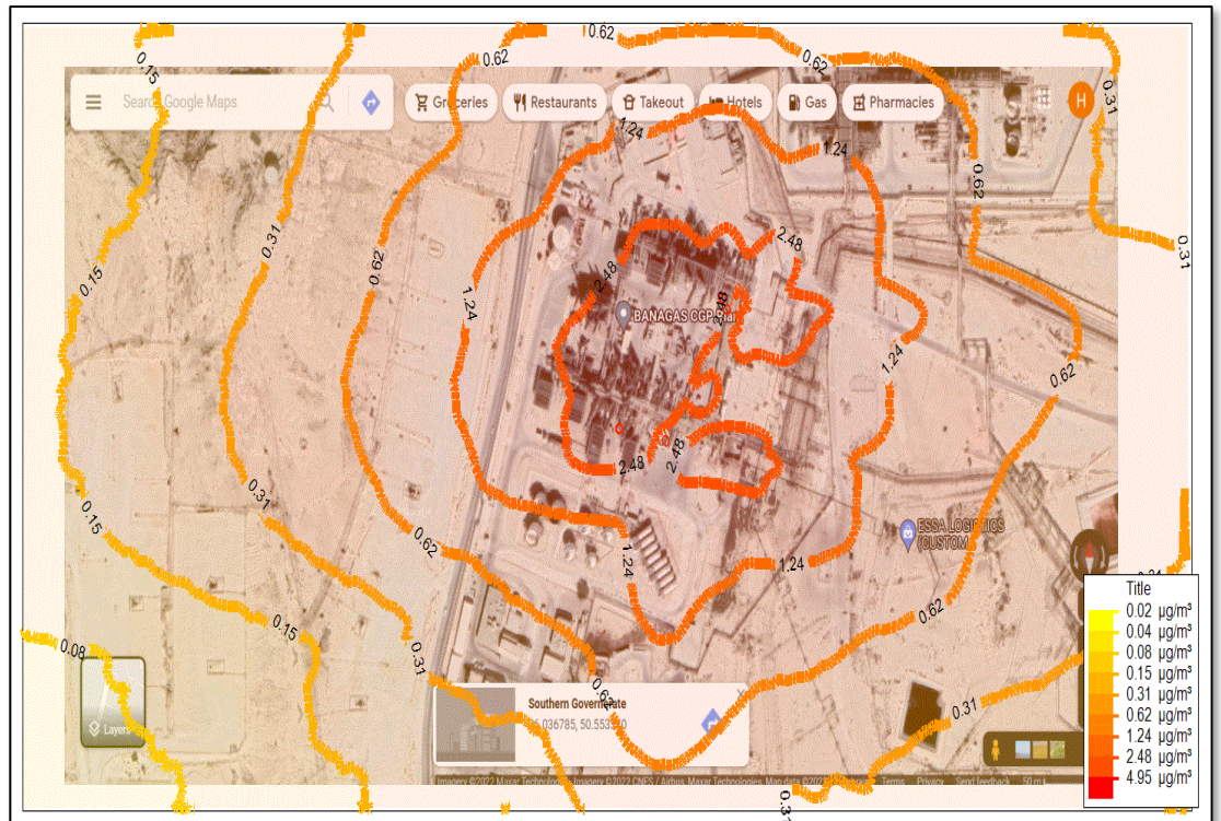
Fig.31: Contours of H 2 S daily maximum concentrations ( \mu\text{g}/\text{m}^3 ) at 6 meters height above the ground- drain pots
