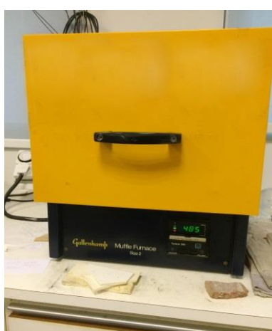
Figure 3.2: The gel was flash sintered in a furnace at 600^{\circ}\text{C} for 1 hour.
