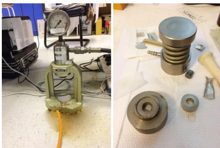
Figure 3.3: The resulting powders were pelletized using Manual hydraulic press.
