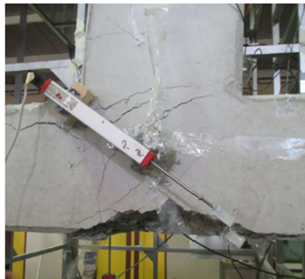
Figure 2.18 Failure of the control sample (Ercan et al., 2019)
