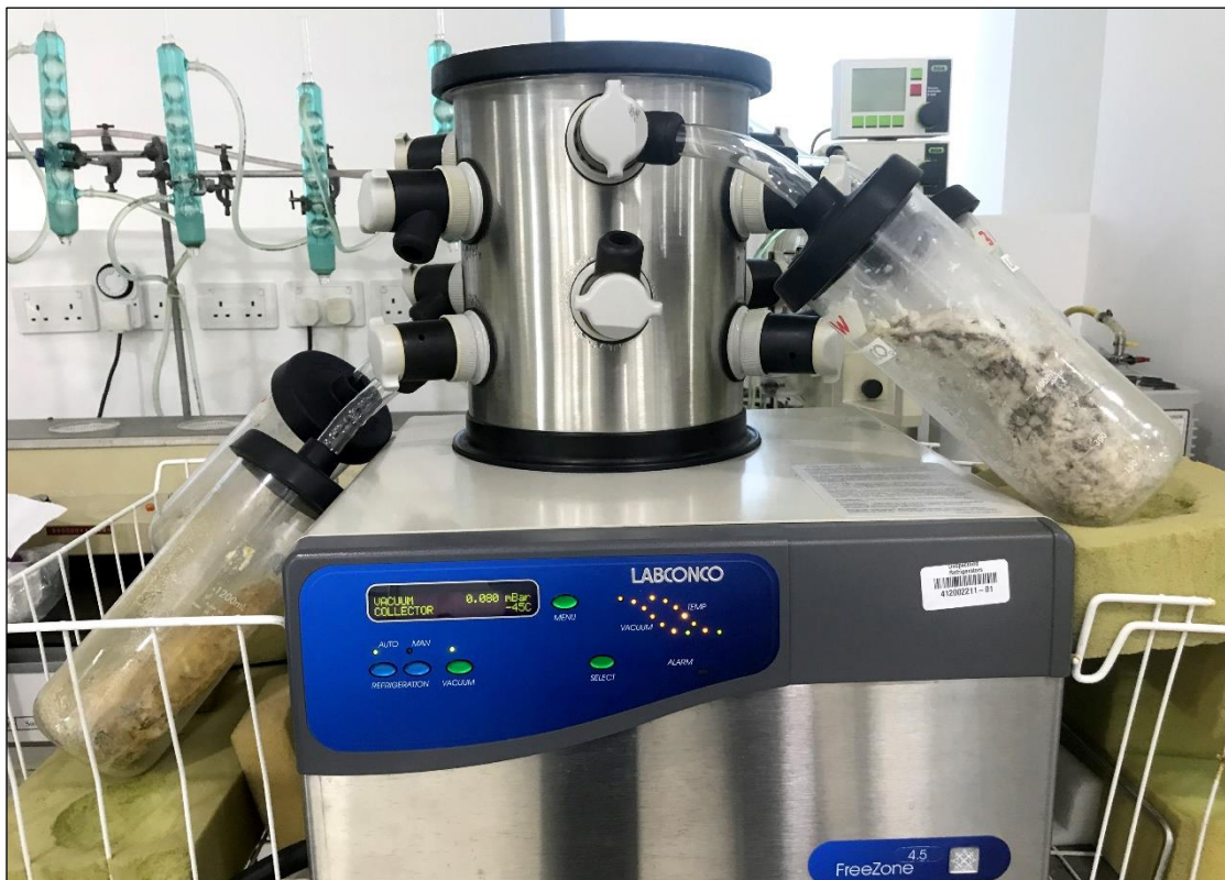
Figure 13 Drying the crab tissues using LABCONCO FreeZone 4.5 freeze dryer.
