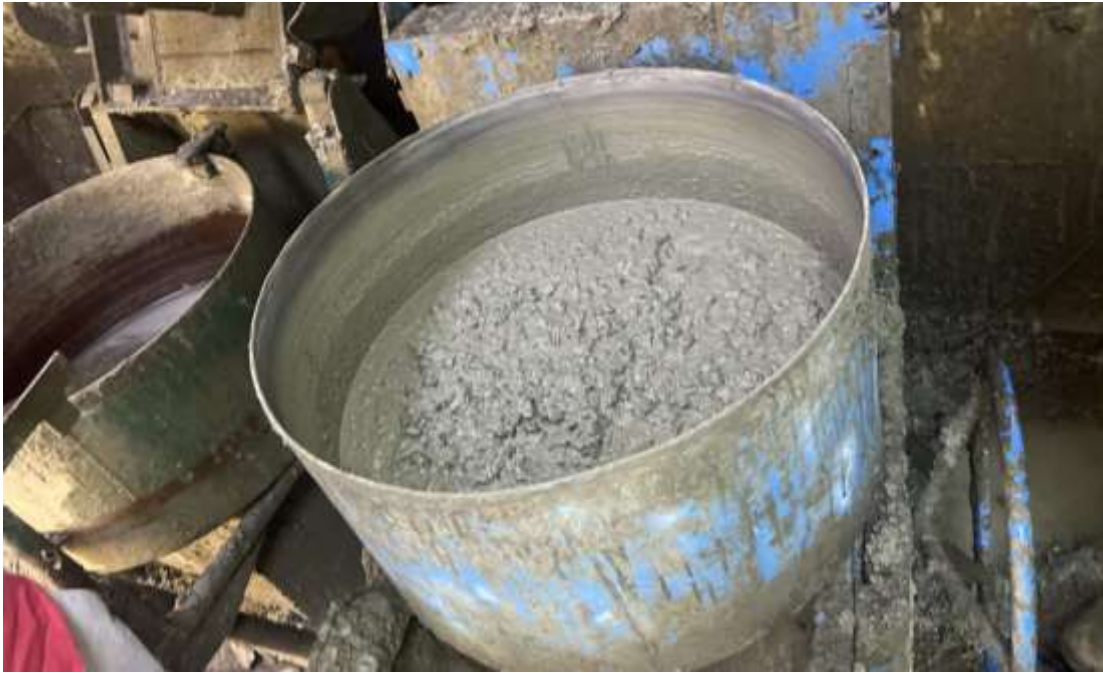
Figure (3. 4): Concrete Mixer with 0.035 m 3 volume
