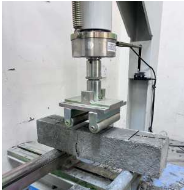
Figure (4. 13): Flexural Strength for the sample with waste money fibers
