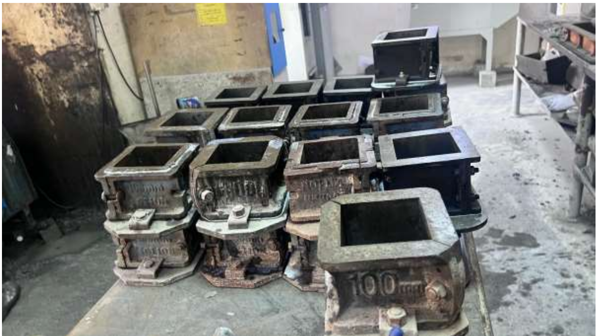
Figure (3. 5): Concrete Molds
