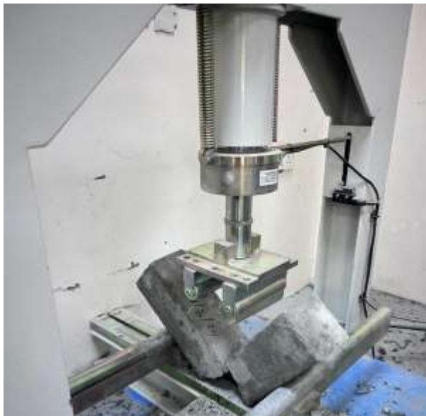
Figure (4. 14): Flexural Strength for the Control Mix
