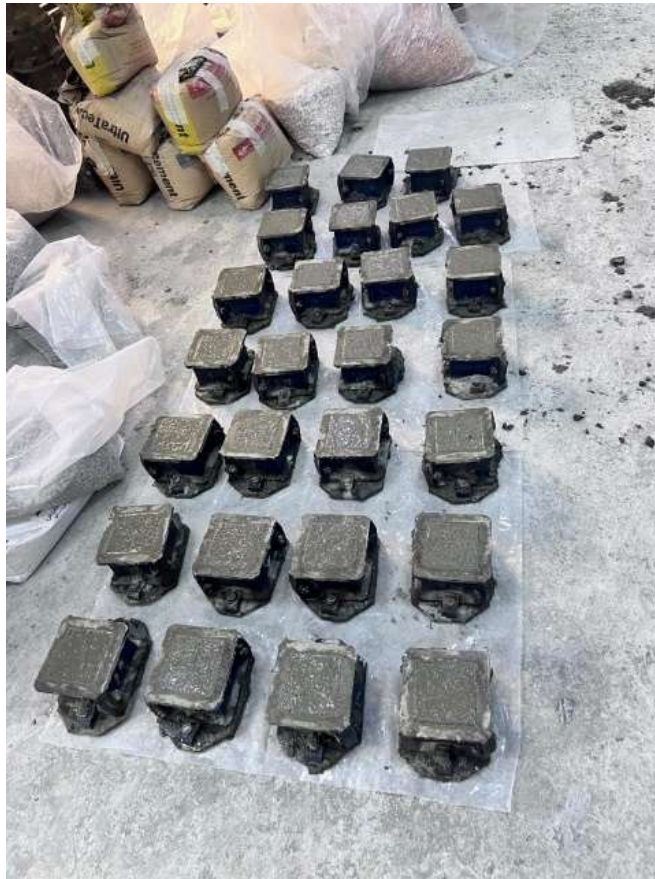
Figure (3. 6): Concrete Cubes for testing
