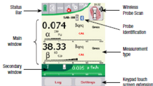
Figure 1: Colibri screen with external alpha/beta probe connected
