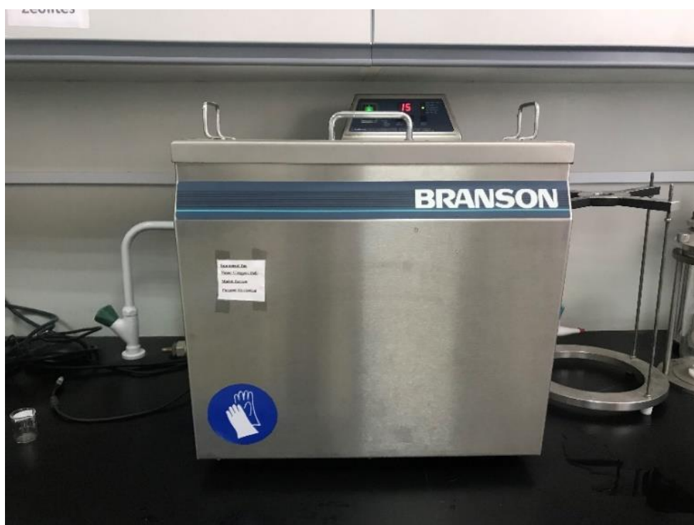
Fig. (A8.2): Ultrasonic bath used for fuel with waxes
