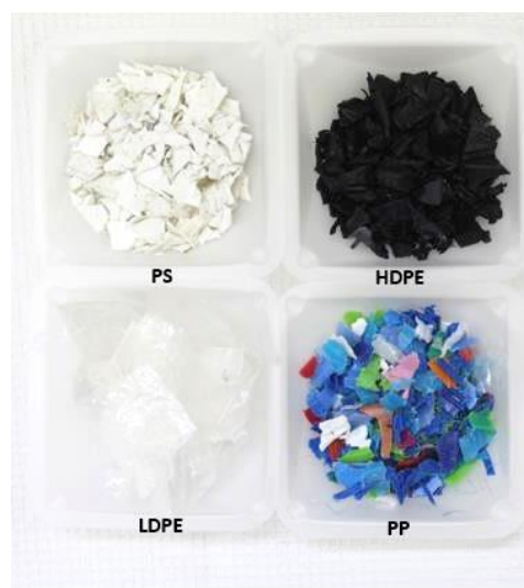
Fig. 26: Sample of waste plastics used
