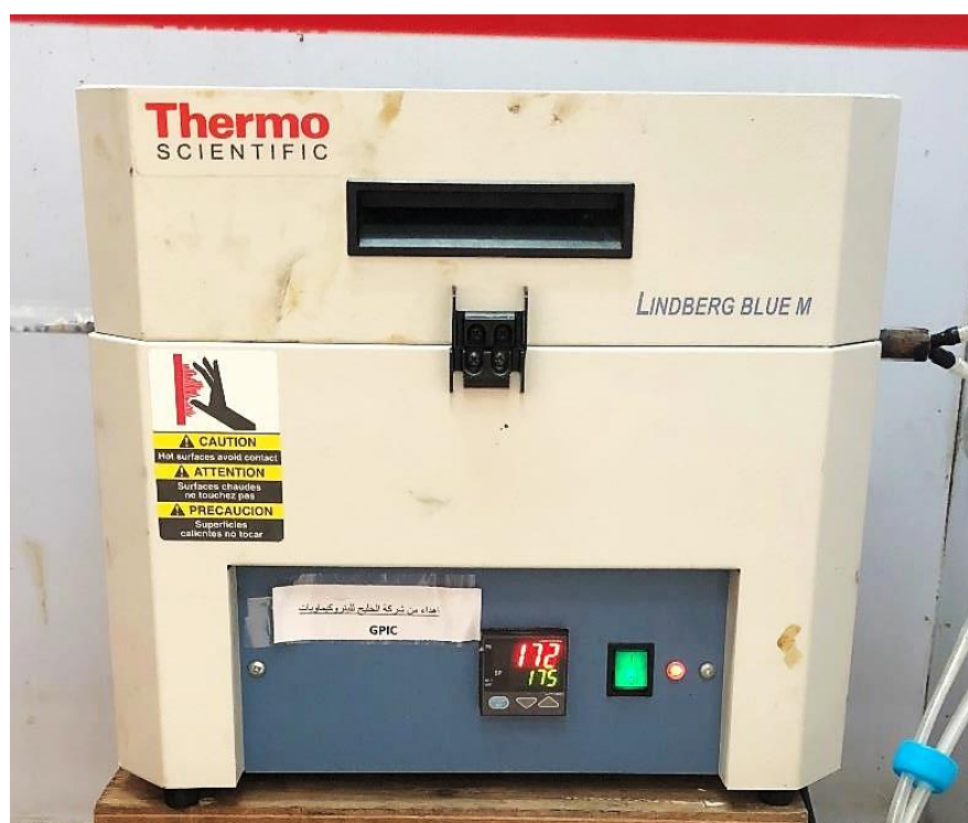
Fig. 31: Glass tube furnace with single set point controller.
