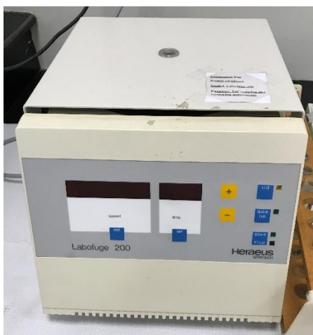
Fig. (A8.3): Centrifuge used for mixing n-hexane with waxes
