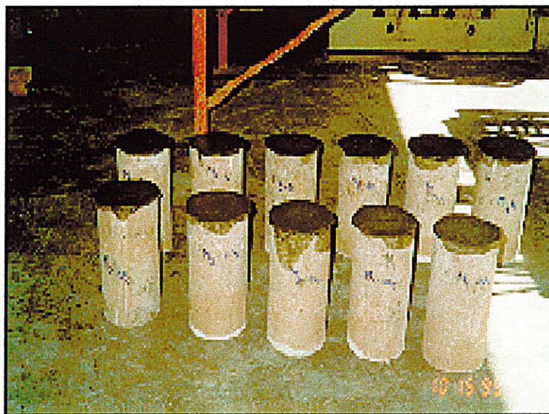
Fig. 3.3. Capping of cylinders
