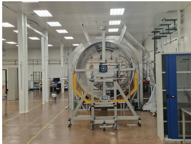
Figure 2.5: MTD Barrel frame where trays will be fitted
