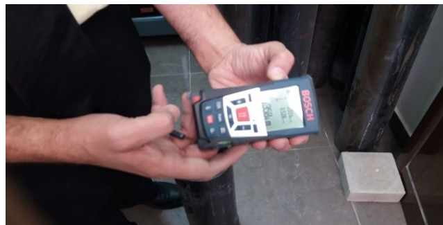
Figure 4-5 Bosch laser EDM that used to measure depth inside pipes
