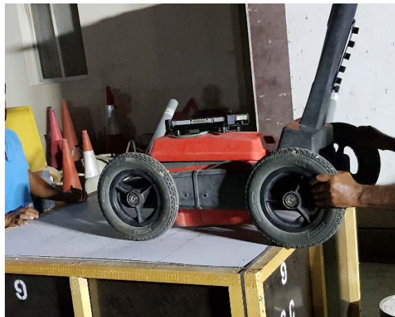
Figure 3-18 GSSI Utility scan – time pulsed dual-frequency GPR
