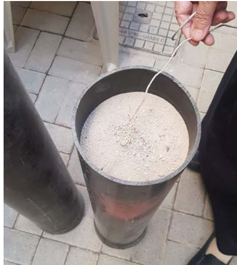
Figure 4-4 Removing the digital sensor from the sample in pipe # 3 (Captured on 06/01/2020)
