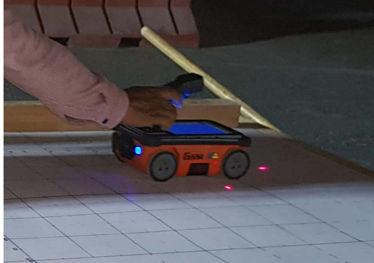
Figure 3-11 GSSI Structscan mini GPR (time domain pulse radar)
