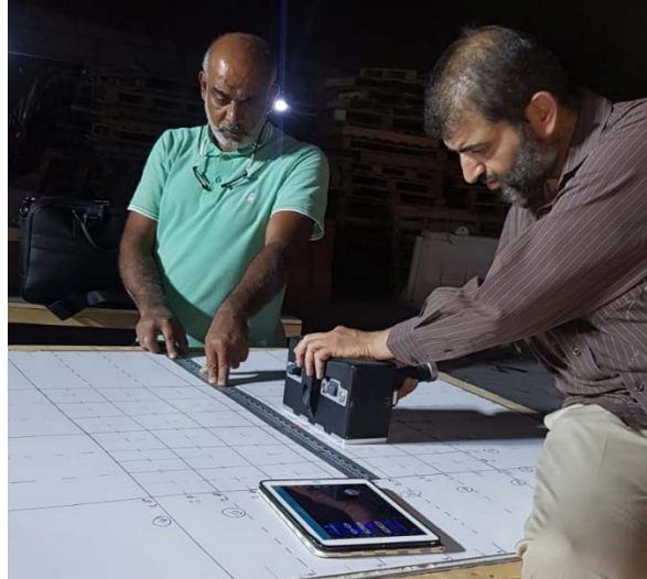
Figure 3-15 Proceq ultrasound (Pundit Array) during data acquisition
