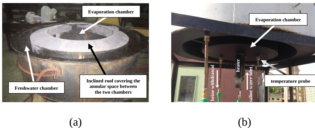
Figure 4.3: Photos of the evaporation chamber (a) top view of the evaporation chamber (without roof), and (b) view from the bottom of the evaporation chamber showing the heater and pipe connections
