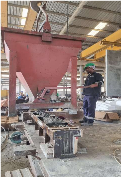
Figure 3.6: Beams Concreting process: (a) concrete batching, (b) concrete pouring using a bucket, (c) surface leveling and vibration, (d) completed beam after casting
