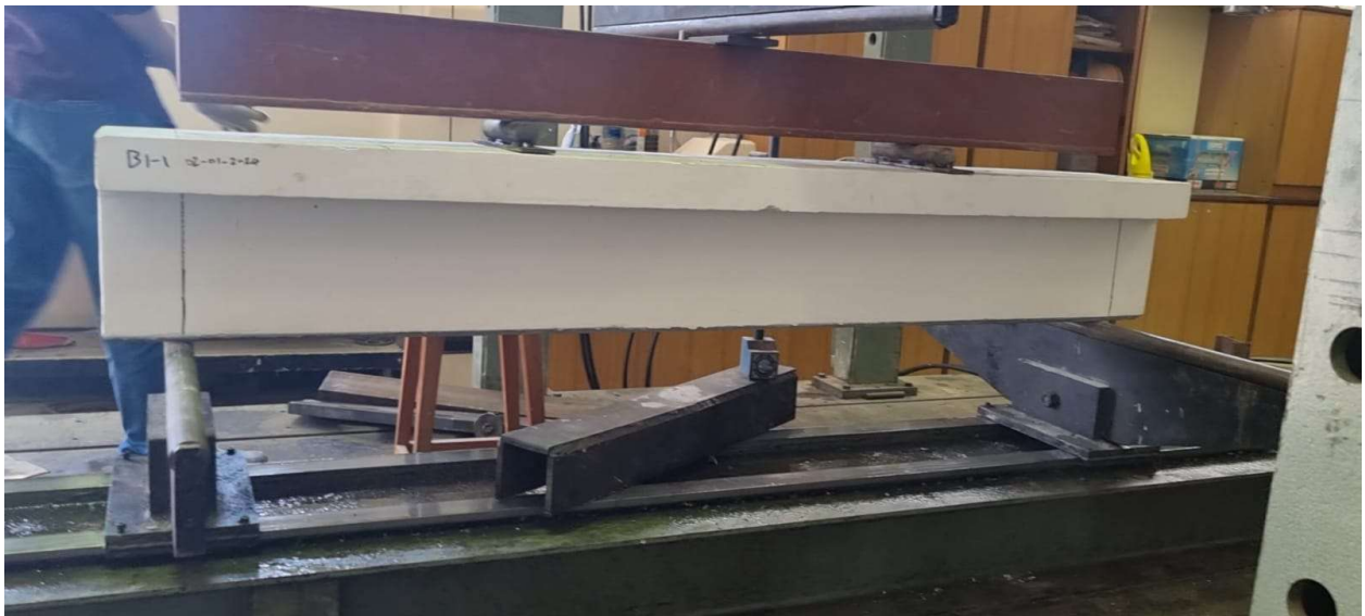
Figure 3.11: Test set up of specimen with a/d of 2 (Lab photograph)
