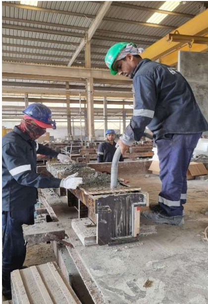
Figure 3.6: Beams Concreting process: (a) concrete batching, (b) concrete pouring using a bucket, (c) surface leveling and vibration, (d) completed beam after casting
