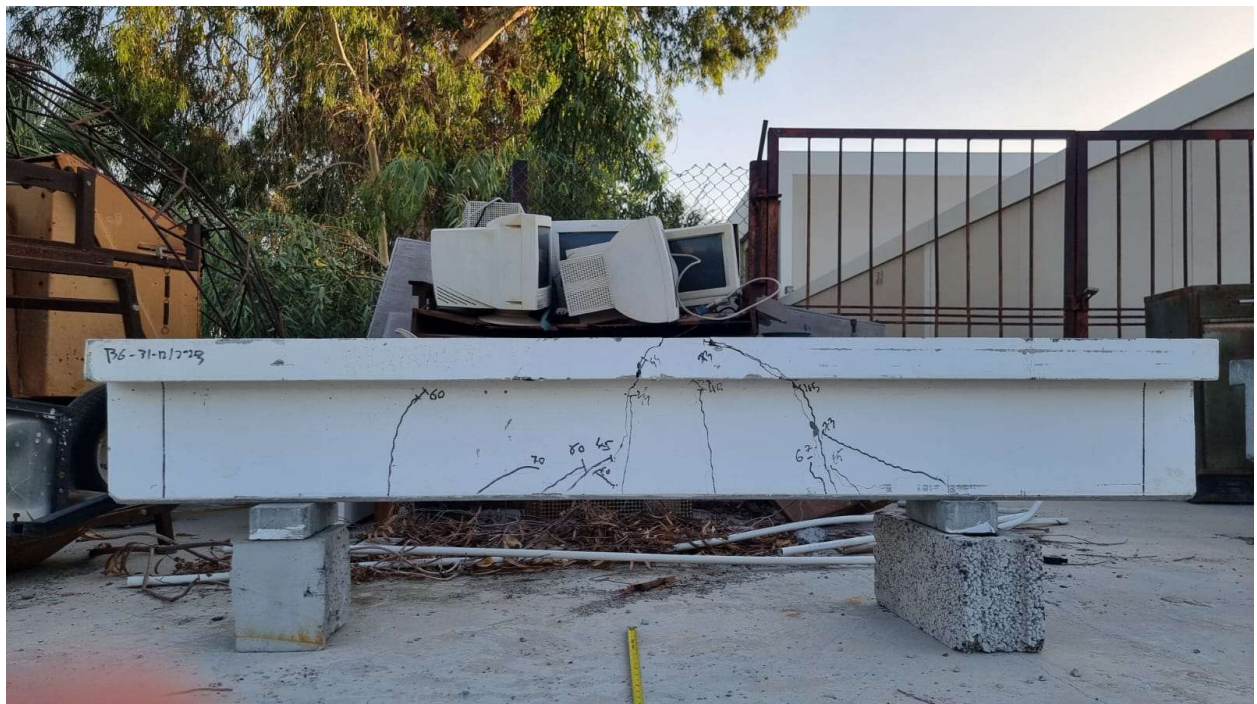
Figure A2. 4: Crack pattern of beam GT-3.5-50-19
