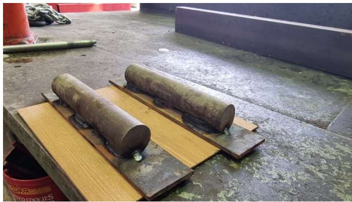
Figure 3.10: Cylindrical steel bars welded to steel plates
