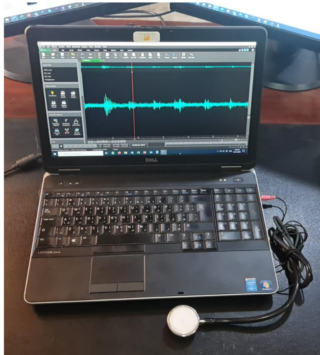
Figure 15: Stethoscope modified for data recording
